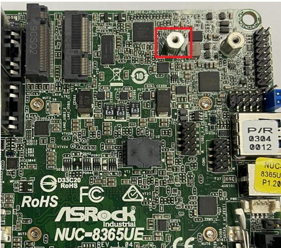
3. Install M.2 2242 storage into the slot, and lock it.
