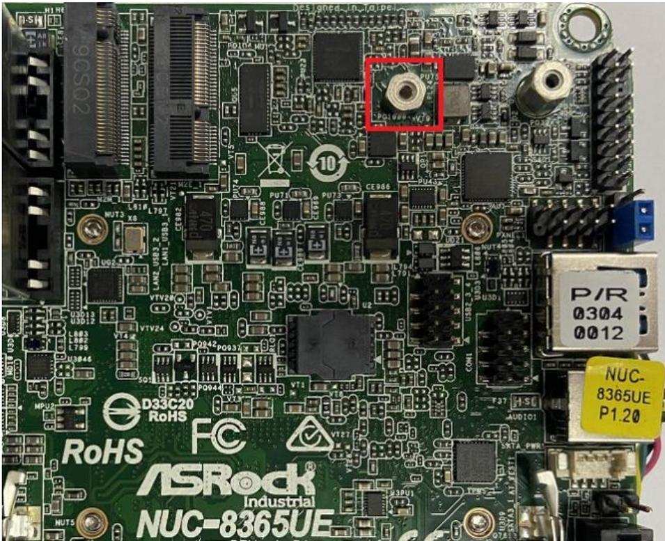
2. Fasten the 6.5 mm standoff into the M.2 Key M 2242 screw hole as following location.
